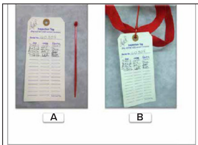
Figure 7: (A) Pull Tie and Inspection Tag (B) Pull Tie and Inspection Tag binding the handles together.
