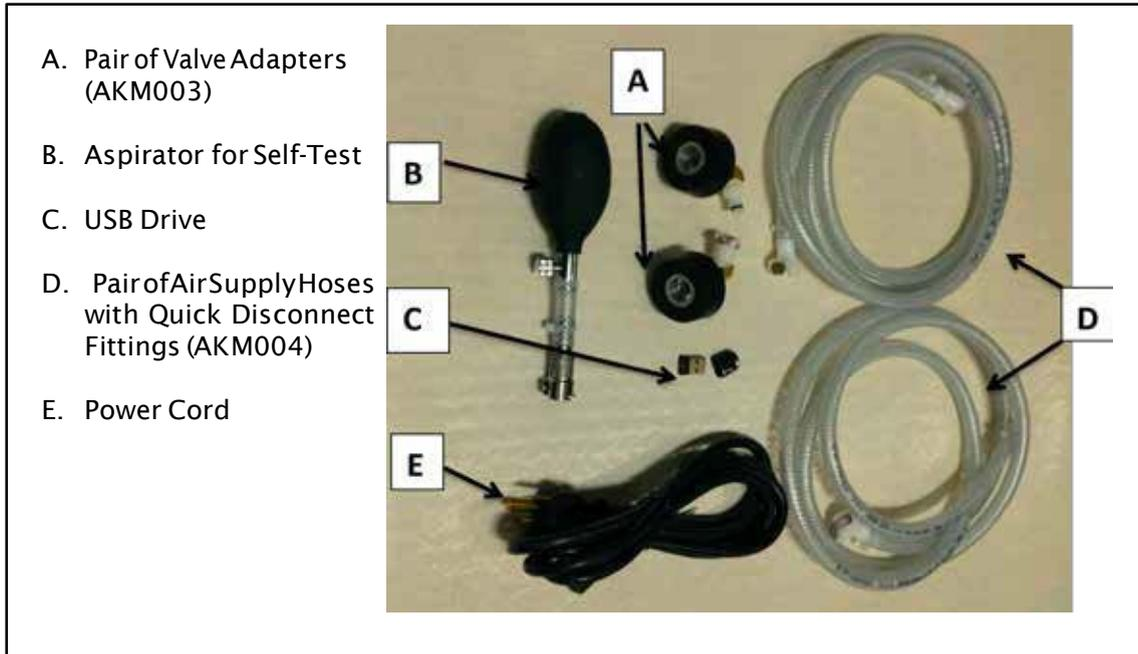
Figure 1: Labeled Components
