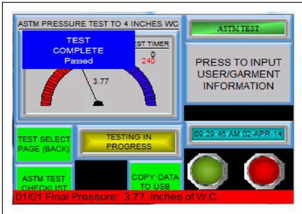
Figure 11: End of Test Output Display
