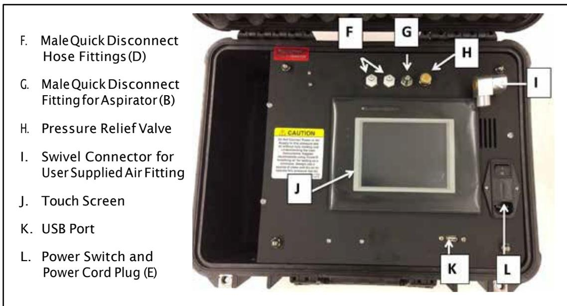
Figure 2: Test Kit Layout
