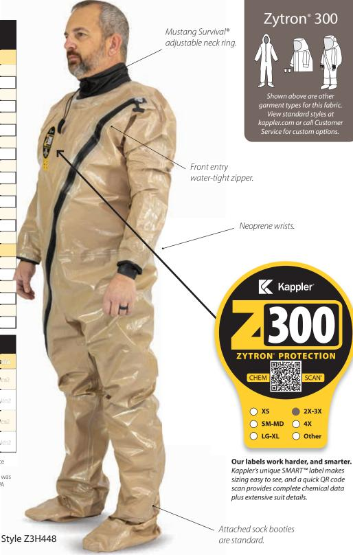
**LIMITATIONS OF USE:** The Z3H448 Wade Suit is intended for initial floodwater approach and entry in response to situations where the potential for contaminated floodwater exists. This garment is not equivalent to a wet suit, dry suit, or dive suit, and provides NO thermal insulation to the wearer. This garment features attached sock booties, which are designed to be worn INSIDE protective footwear ONLY.
