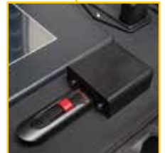
The built-in USB port allows easy connection to a data storage device.
