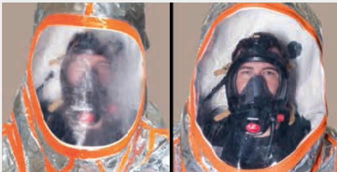
Comparison shows Standard Visor vs. AntiFog Visor.
