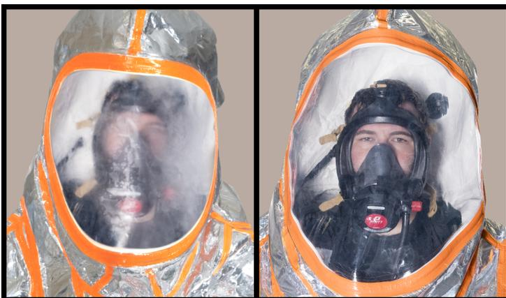
*Unretouched images show standard visor on left after only a few minutes in suit. Right image shows Kappler's AntiFog Expanded View Visor after 30 minutes of wear.*
